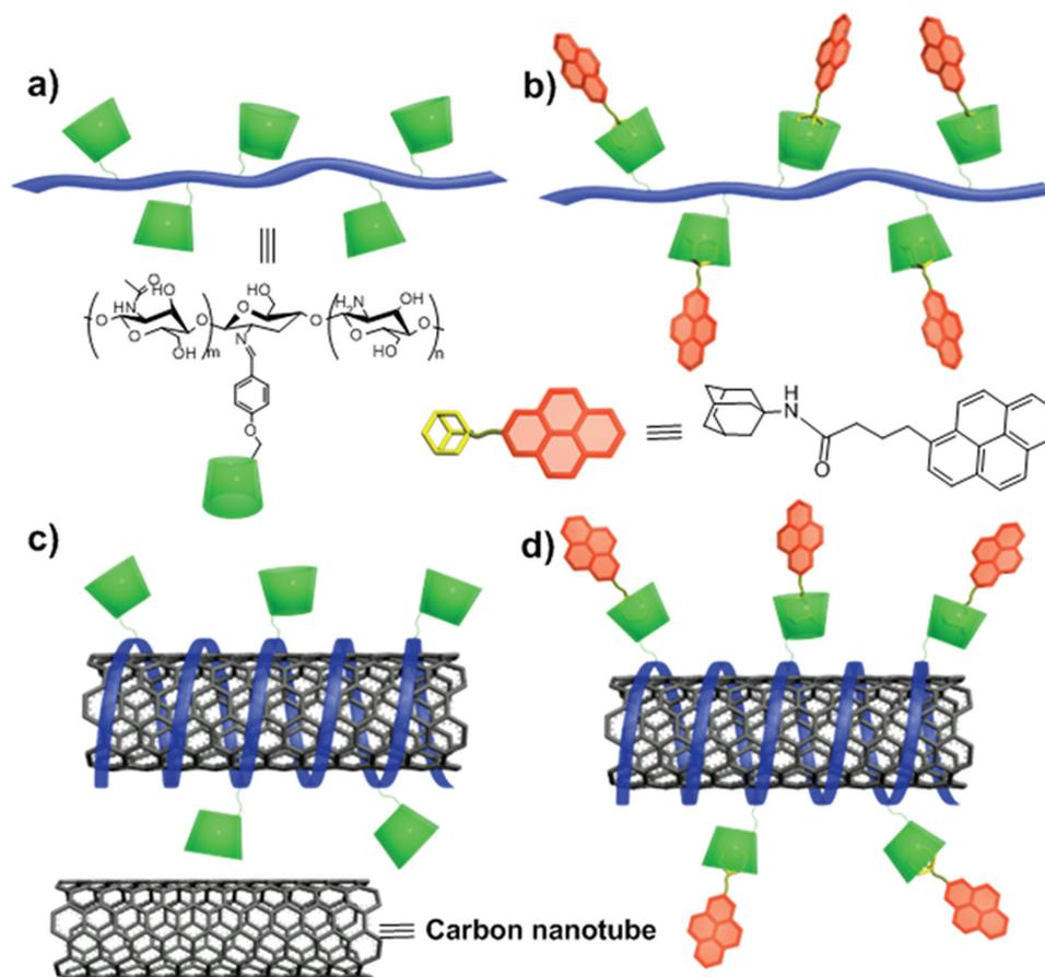
**Figure 3.** Secondary assemblies of CD-grafted chitosan/adamantanyl pyrene with carbon nanotubes in different sequences: a) CD-grafted chitosan, b) CD-grafted chitosan/adamantanyl pyrene dyad assemblies, c) CD-grafted chitosan/carbon nanotube dyad assemblies, d) CD-grafted chitosan/carbon nanotube/adamantanyl pyrene triad assemblies.
