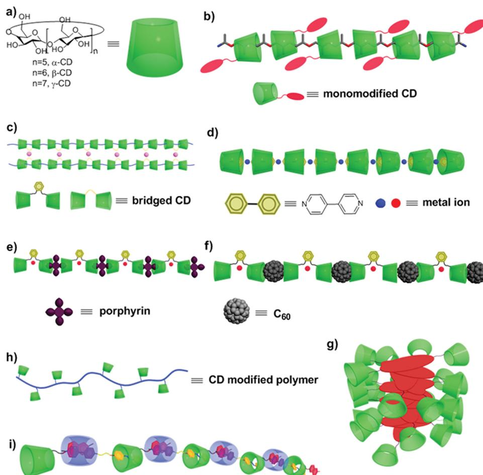
**Figure 1.** Schematic illustration of: a) CDs; b,c) CD-based 1D supramolecular strand with covalent polymer as the core; d) CD-based 1D strand with coordinated polymer as core; e) CD-based 1D strand with polyporphyrin as the core; f) CD-based 1D strand with polyfullerene as the core; g,h) self-assembled 1D supramolecular strand, and i) 1D supramolecular strand with CD grafts.
