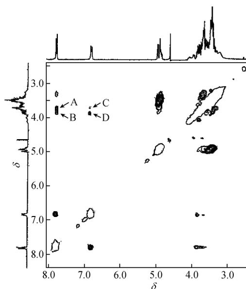
Fig. 4. <sup>1</sup>H ROESY spectrum (300 MHz) of **1** ( $[1] = 1.0 \times 10^{-3}$  mol/L) in D<sub>2</sub>O at 298 K with a mixing time of 300 ms.
