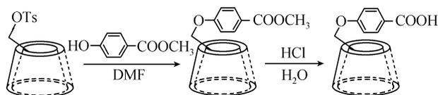
Fig. 1. The synthetic route of compound **1**.
