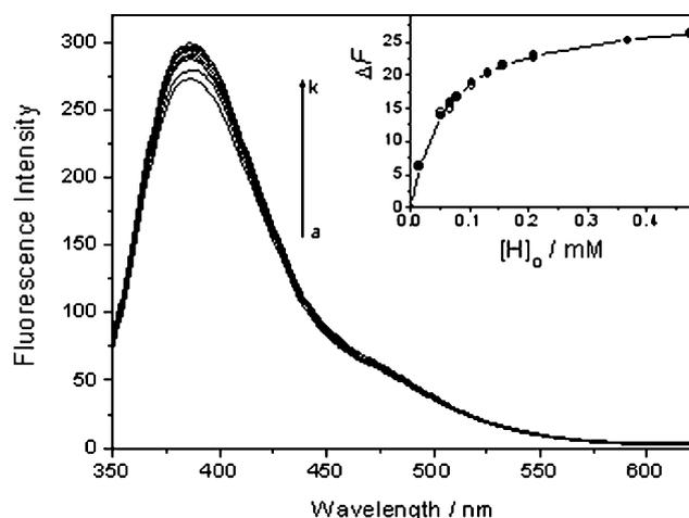
Fig. 2 Fluorescence spectral changes of CID (0.007 mM) upon addition of DM $\beta$ CyD (0–0.49 mM from *a* to *k*) at pH 1.5 and the nonlinear least-squares analysis (inset) of the differential intensity ( $\Delta F$ ) to calculate the complex stability constant ( $K_s$ ). The excitation wavelength is 329 nm.
