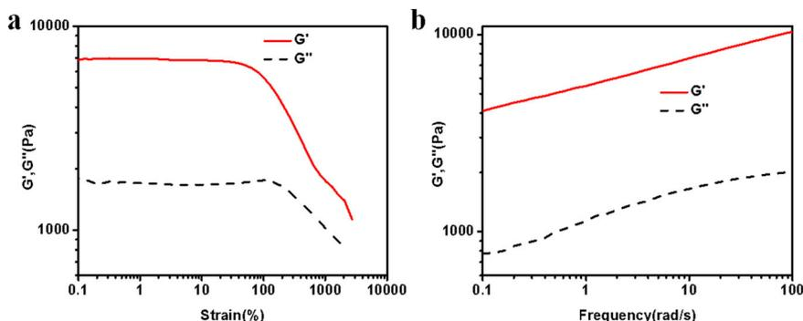
**Fig. 3** Rheological characterization of the hydrogel. **a**  $G'$  (storage modulus) and  $G''$  (loss modulus) as functions of strain. **b**  $G'$  and  $G''$  as functions of frequency (ACA-PEG<sub>20000</sub>-ACA: Hy- $\alpha$ -CD = 1:5).
