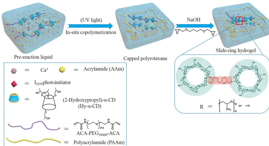
**Fig. 1 Schematic illustration.** Construction of Hy- $\alpha$ -CD/ACA-PEG<sub>20000</sub>-ACA/Ca hydrogel. (Formation of capped polyrotaxane by photopolymerization; formation of slide-ring hydrogel through further cross-linked cyclodextrins).
