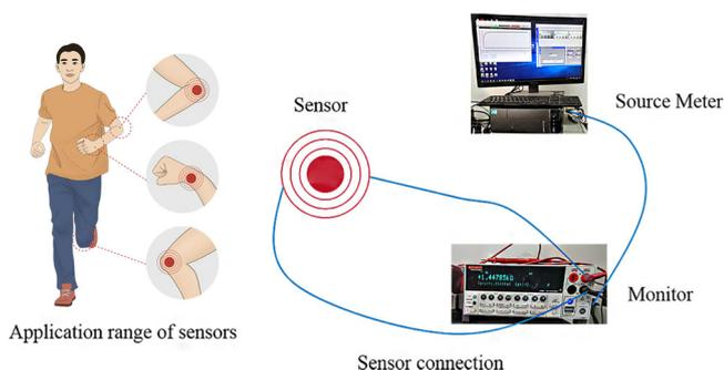
**Fig. 7 The sensing application of strain sensors and the composition and signal conversion process of strain sensors.** After receiving the human motion signal, the sensor is monitored by the detector (monitor; source meter), and then processed by the processor (computer) and converted into a digital signal.
