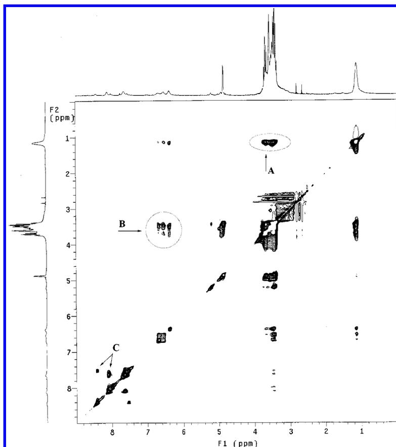
**Figure 10.**  $^1\text{H}$  NOESY spectrum (300 MHz) of a mixture of **2**-Ni(II) with RhB ( $[\text{2-Ni(II)}] = [\text{RhB}] = 5.0 \times 10^{-4} \text{ mol dm}^{-3}$ ) in  $\text{D}_2\text{O}$  at 298 K with a mixing time of 800 ms.
