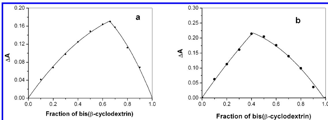
**Figure 3.** Continuous variation plot of (a) **2**/Cu(II) ( $[\mathbf{2}] + [\text{Cu}^{2+}] = 1.1 \times 10^{-4} \text{ mol dm}^{-3}$ ) and (b) **3**/Cu(II) system. ( $[\mathbf{3}] + [\text{Cu}^{2+}] = 1.5 \times 10^{-4} \text{ mol dm}^{-3}$ ).
