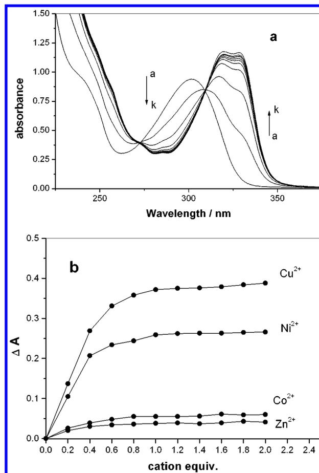
**Figure 1.** (a) UV-vis spectral change of **2** upon addition of copper(II) ion in aqueous solution. ( $[2] = 1.5 \times 10^{-4} mol dm^{-3}$ ,  $[Cu^{2+}] = 0-3.0 \times 10^{-4} mol dm^{-3}$  from a to k) (b) spectrophotometric titration of **2** at 302 nm with four metal ions in aqueous solution. ( $[2] = 1.5 \times 10^{-4} mol dm^{-3}$ ; counteranion:  $NO_3^-$ ).
