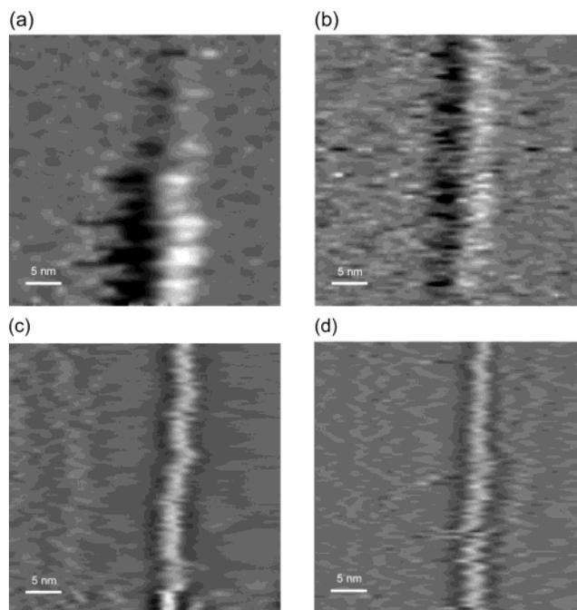
**FIGURE 5.** Series of STM images of compound **2** at (a) 0, (b) 9, (c) 16, and (d) 24 min illustrating Ostwald ripening.  $I_t = 2.1$  nA,  $V_b = 300$  mV.
