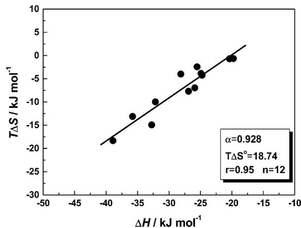
**Figure 3.** Enthalpy–entropy compensation plot for the inclusion complexation of various bile salts with aminated  $\beta$ -CDs **2**–**4** obtained in the present work in aqueous buffer solution at 298.15 K.
