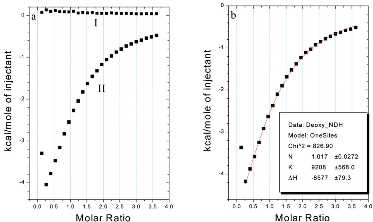
**Figure 2.** (a) Heat effects of dilution (I) and of complexation (II) of **4** with DCA for each injection during titration microcalorimetric experiment. (b) "Net" heat effect obtained by subtracting the heat of dilution from the heat of reaction, which was analyzed by computer simulation using the "one set of binding sites" model.
