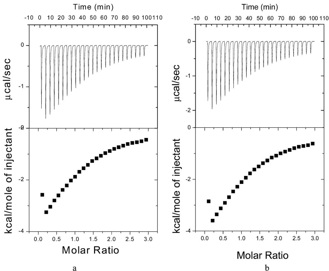
**Figure 1.** Calorimetric titrations of host **2** with CA (left) and DCA (right) in phosphate buffer (pH 7.20) at 25 °C. (a) Raw data for sequential 10  $\mu\text{L}$  injections of CD solution (2.00 mM) into bile salt solution (0.13 mM). (b) Heats of reaction as obtained from the integration of the calorimetric traces.
