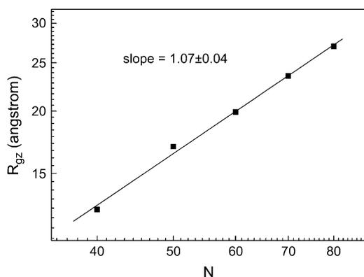
Fig. 2. Log–log plot of  $R_{g_z}$  of alkane molecules in SWCNT(9,9) as a function of chain length  $N$ .
