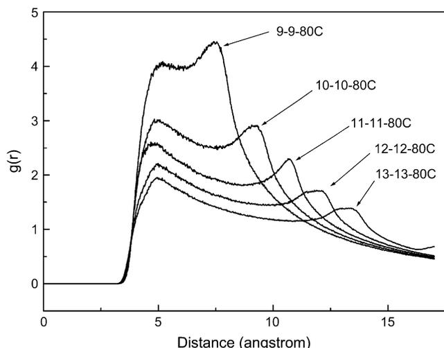
Fig. 3. Radial distribution function  $g(r)$  of  $C_{\text{CNT}}-C_{\text{alkane}}$  for 9-9-80C, 10-10-80C, 11-11-80C, 12-12-80C, and 13-13-80C.
