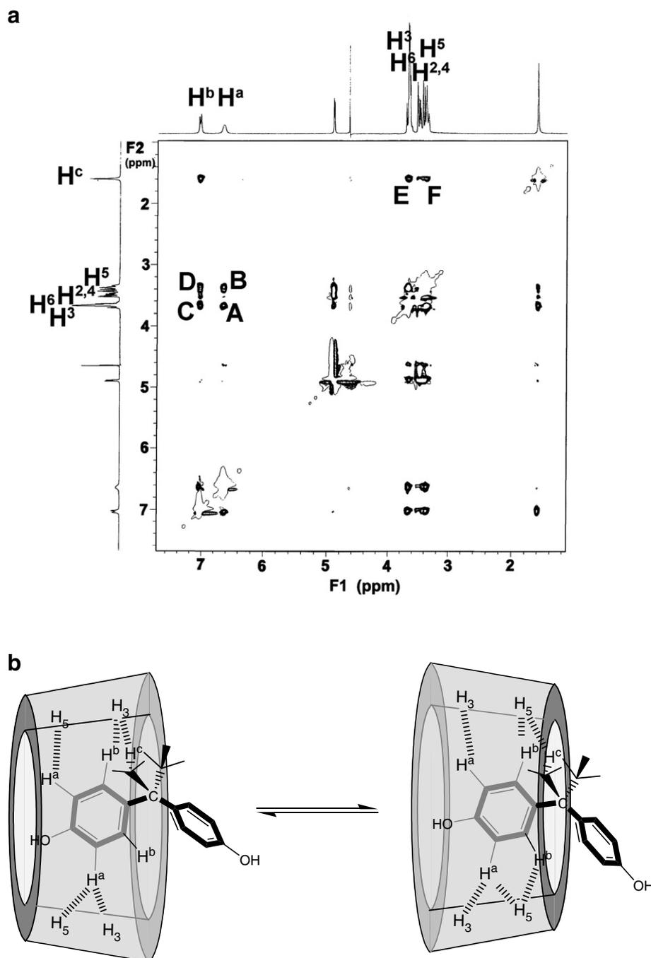
**Figure 3.** (a) <sup>1</sup>H ROESY spectrum of the  $\beta$ -CD/BPA complex ( $8 \times 10^{-3}$  mol L<sup>-1</sup>) in D<sub>2</sub>O at 25 °C with a mixing time of 200 ms. (b) Possible structure of the complex in aqueous solution.
