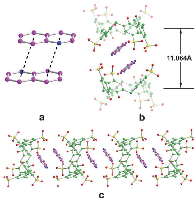
**Fig. 5** View of the QU dimer (a), the sandwich unit formed by the two half-C6AS (shown in opaque) and one dimer (b) and the structure of the polymeric sandwich complexes along the crystallographic  $a$  direction in complex **3**.
