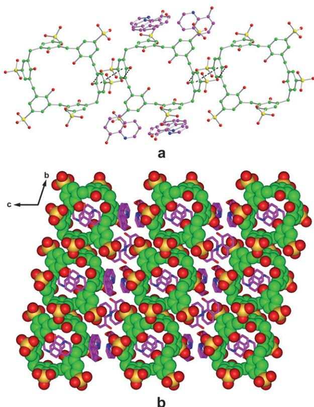
**Fig. 8** View of the host molecule environment in a hydrophobic layer (a) and the multipillar aggregate of complex **4** in the crystallographic  $b \times c$  plane (polymeric sandwich complexes running perpendicular to the plane of the page) (b).
