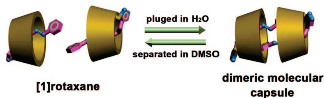
FIGURE 3. Structural transformation of 1 by changing solvents.
