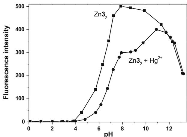
**Figure 3.** Fluorescence intensities of Zn·3<sub>2</sub> (10 μM) in the absence and presence of Hg<sup>2+</sup> (10 μM) at various pH values in aqueous solution at 298 K ( $\lambda_{\text{ex}} = 352$  nm,  $\lambda_{\text{em}} = 500$  nm).
