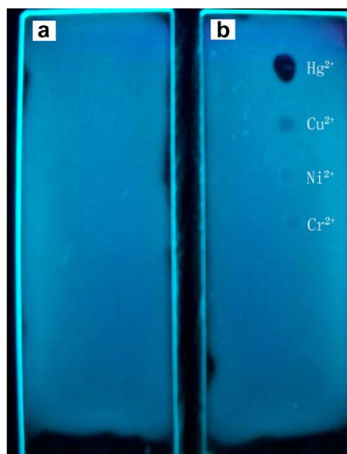
**Figure 5.** Images of Zn·3<sub>2</sub>-contained PVA film in the absence (a) and (b) presence of metal ions under the low intensity UV light ( $\lambda = 360$  nm).
