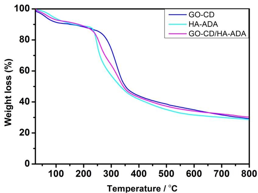
**Fig. S4.** TGA curves of GO-CD, HA-ADA, and GO-CD/HA-ADA complex, respectively.
