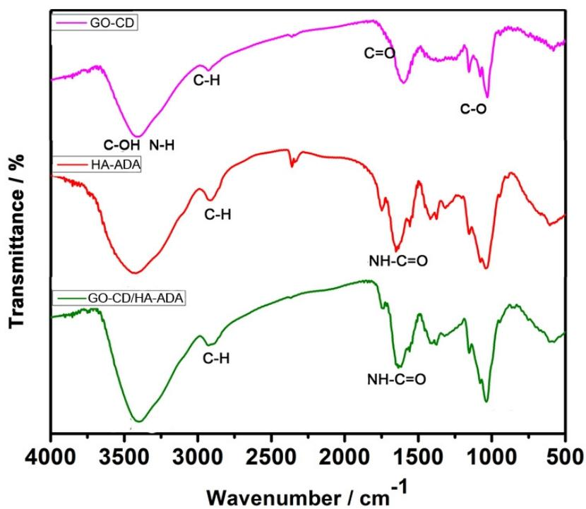
**Fig. S3.** FTIR spectra of GO-CD, HA-ADA, and GO-CD/HA-ADA complex, respectively.
