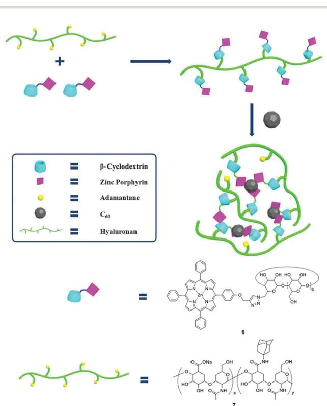
**Scheme 1** Construction of polysaccharide–porphyrin–fullerene supramolecular conjugates.
