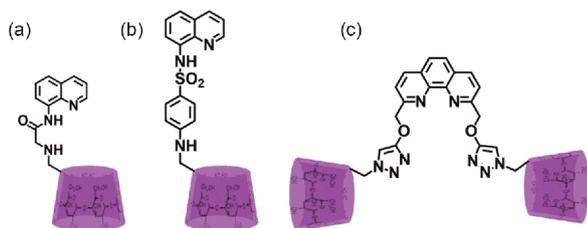
**Figure 2** Molecular structures of  $\beta$ -CDs modified by (a) 8-aminoquinoline, (b) *N*-(8-quinolyl)-*p*-aminobenzenesulfonamide (HQAS), and (c) 1,10-phenanthroline for the detection of  $\text{Zn}^{2+}$  in water (color online).
