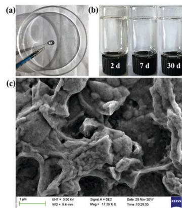
**Fig. 3** (a) Illustration of the injectability of the hydrogels. (b) Photographs at different time intervals after gelation at r.t. (c) SEM images of the supramolecular hydrogels (CNSs/PPR 2 = 2.4/0.097 wt%), and the scale bar in SEM image is  $1 \mu\text{m}$ .
